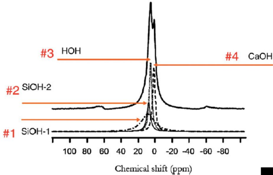
Magic Angle Spinning Spectroscopy.  $\text{C}_3\text{S}$  hydrated one year. Korb, Current Opinion Colloid Interface Science, 2009.
