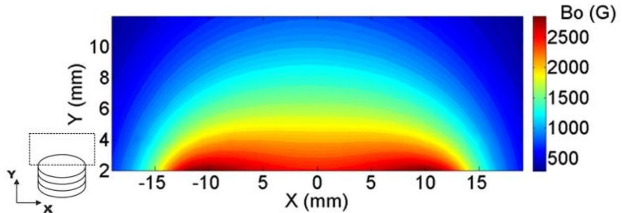
Linear gradient from 2–7 mm above magnet, 2000 Gauss/cm.
