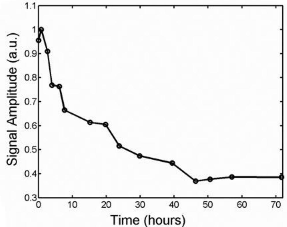
Curing mortar (w/c = 0.45). Avg. first 2 echoes, 8192 avg.
