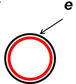
Assumes rapid exchange of bound water surface layer and bulk water in pore centre.  $S/V$  is pore size. 'Solid'  $^1\text{H}$  not observed.
