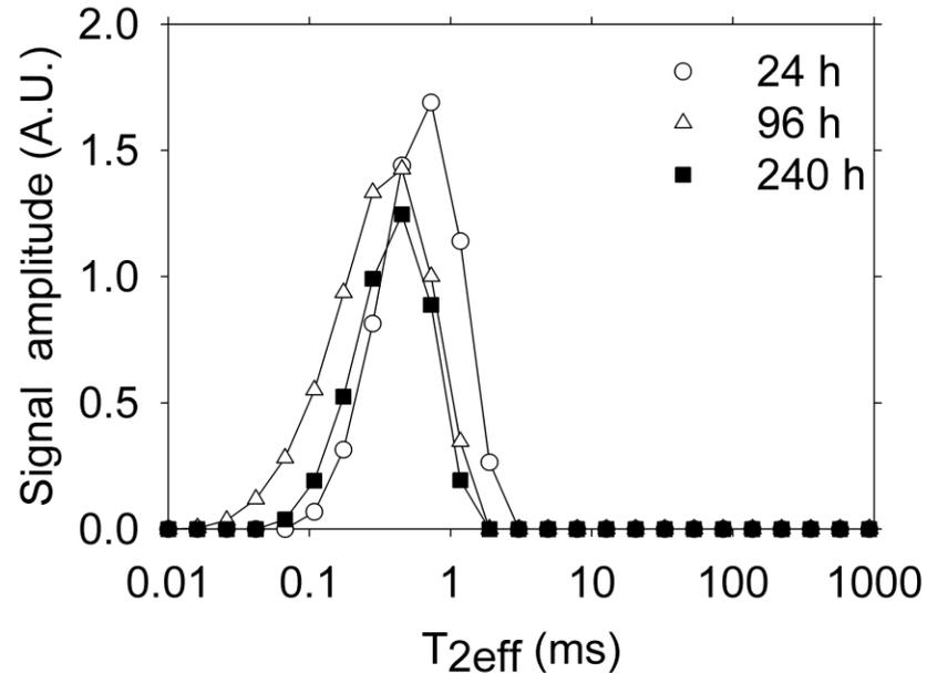
**Embedded magnet  $T_2$  distribution,  $w/c = 0.6$ .**
