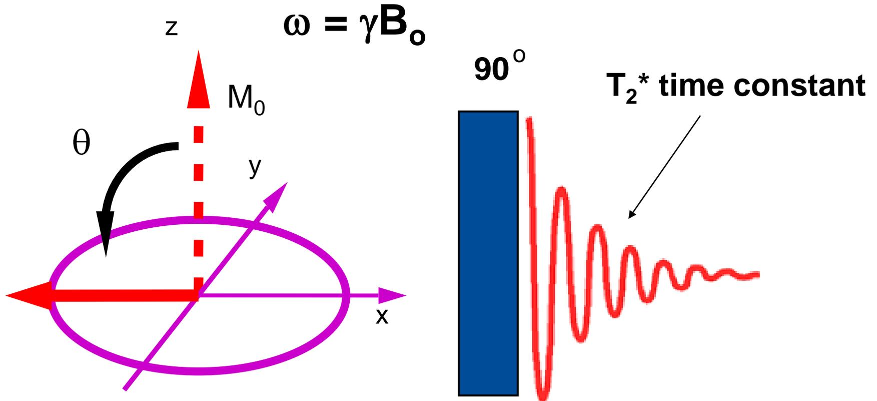
$B_0$  2.4 Tesla, RF signal 100 MHz
