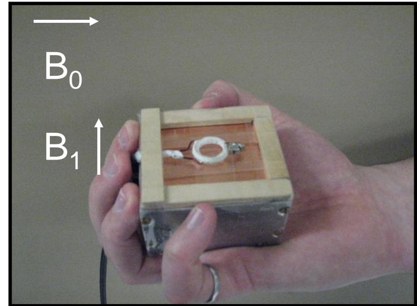
**~ 1 cm<sup>3</sup> spot displaced 0.8 cm from surface, 0.9 kg magnet.**
